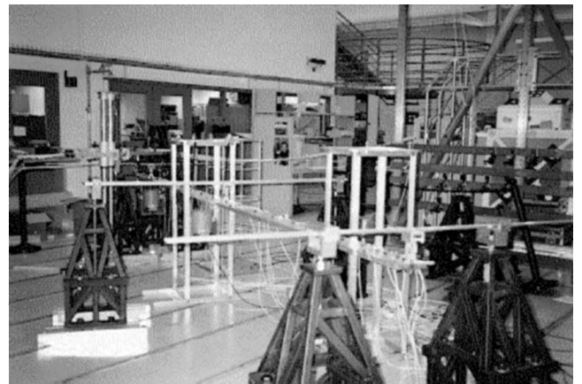
Fig. 4 Overview of modal test setup for component 1 of the free-free beam.
